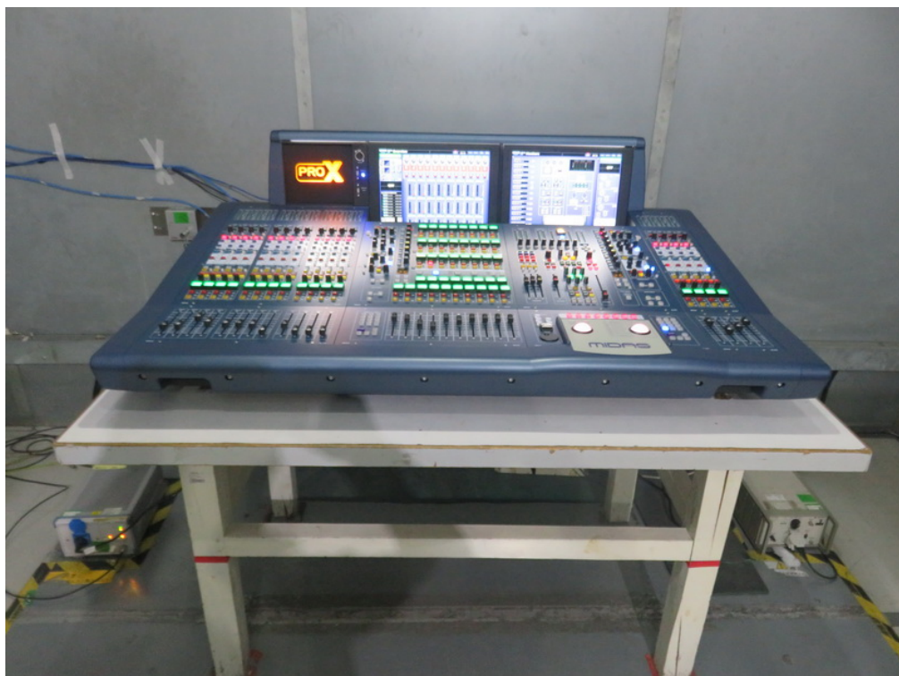
Conducted emissions AC mains power port
